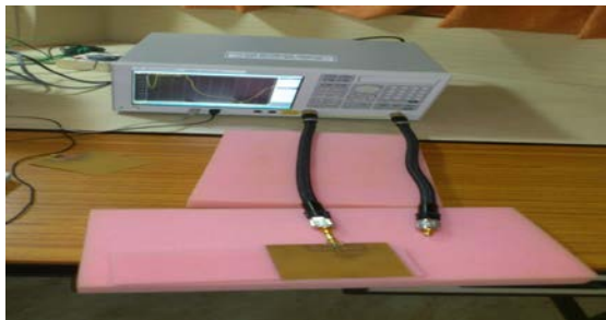
Fig11: a) Proposed antenna testing by using Vector Network Analyzer(E5071C) b) Resonant frequency
