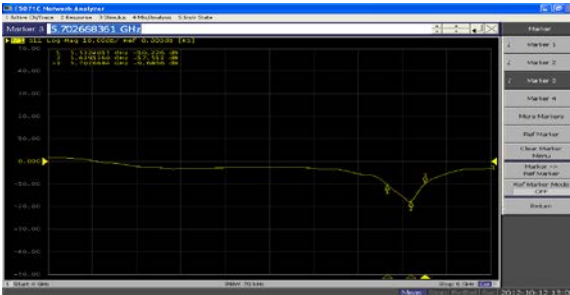
a) Simulated Return loss characteristics (in Ansoft HFSS v12) b) Return loss characteristics by network analyzer for L-Shape
